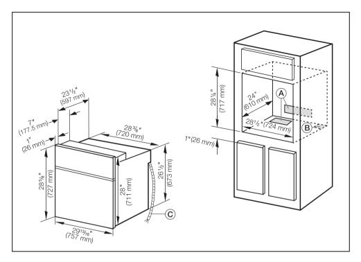
A Vent cut-out (min. 24"<sup>2</sup> / 150 cm<sup>2</sup>) possible at rear or platform of cabinet
